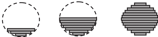
Figure 1.3 Layered manufacturing of an elliptical shape
